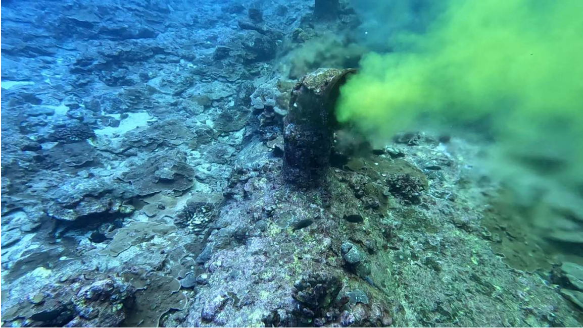
Figure 9. Typical diffuser port with discharge of dye
