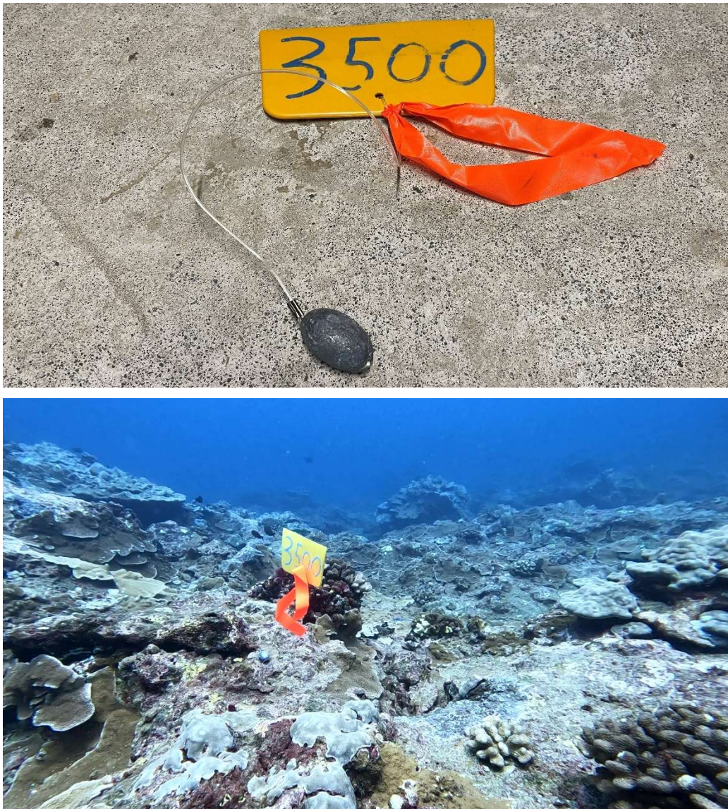
Figure 3. Station marker closeup ( top ) and as deployed on the outfall ( bottom )
