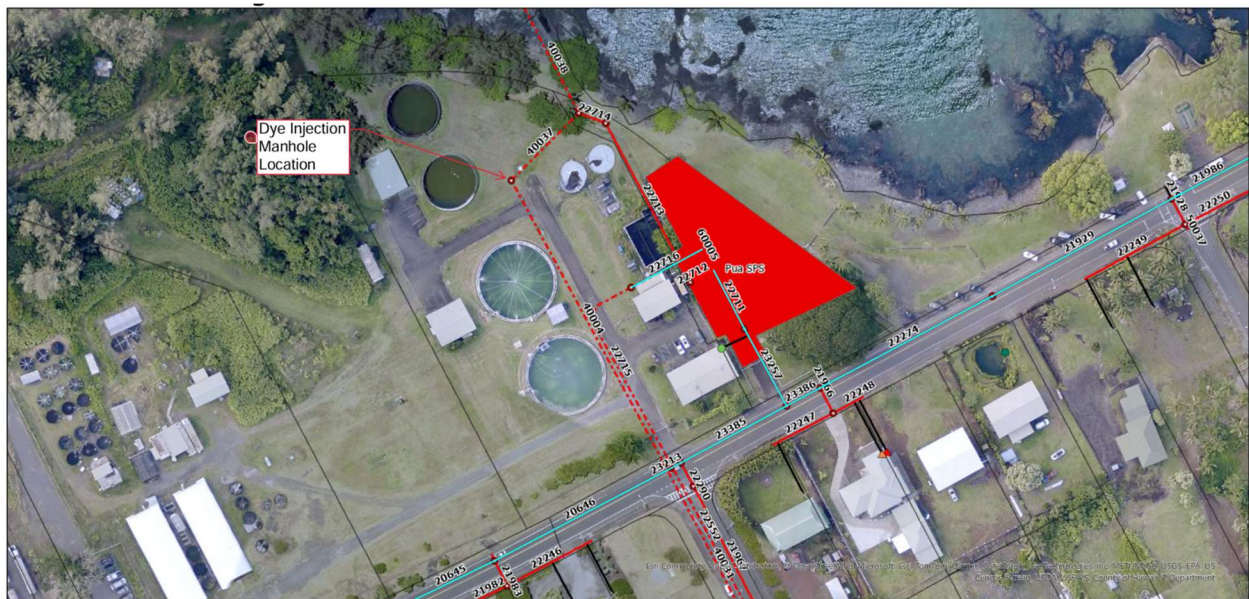
Figure 4. Manhole location used to introduce the tracer dye at Hilo WWTP
